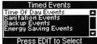
**N.B.** Although event 1 is shown as Inhibit, it is possible for the operator to set event 1 as the first Free Vend or Discounted Vend period.
