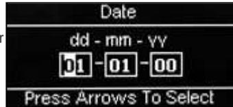
Pressing the ↵ (Edit) key will move back to the Clock menu screen and save the date to the machines memory. Confirm that the status line at the bottom of the screen displays the correct date when Date is highlighted.
