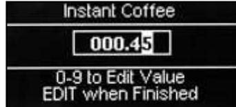
5. Press the ↵ (Edit) key to return to the Individual Prices screen and verify that the new price displays in the status line along the bottom of the display. Use the ▲(up) or ▼(down) keys to highlight further selections.
