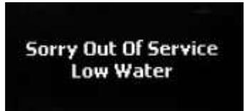
**Note!** The machine has a safety cut-out which will only allow the heater tank to fill for a maximum of two minutes. If after power-up the heater tank has not filled within this time, the mains power supply should be switched off and then on again to reset the heater tank time-out.
