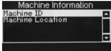
2. When complete, press the **X** (Exit) key to return to the Machine Information menu screen. If necessary press the **▼** (down) then **↵** (Edit) keys to highlight then enter the Machine Location screen. When complete press the **X** (Exit) key.
