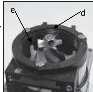
3. Take the new grinder body complete with inner grinder ring from the service kit. Screw the grinder body clockwise into the blade housing until it stops.
