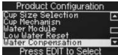
The goal is to vend the programmed amount of water (in Selection Timers) during a vend, more or less will be vended by increasing or decreasing the numeric value. FB Compensation relates to low pressure drinks, Esp Compensation relates to high pressure drinks and is set in exactly the same way.
