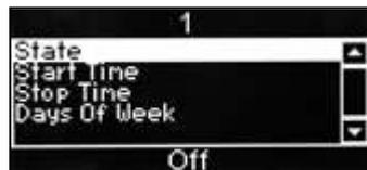
3. Press the ↵ (Edit) key to access the State sub menu. Using the ▼(down) key, set the State to On (indicated by the filled radio button). Press the ↵ (Edit) key to return to the Event 1 screen. Verify that the status line confirms the State is set to On.
