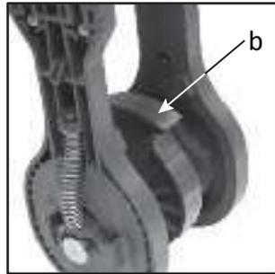
8. Holding the lower piston and cylinder assembly as shown, guide the assembly into the swing arms/filter holder assembly.
