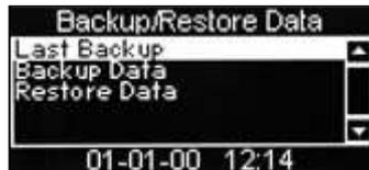
4. To restore the machines memory to the last available backup, scroll down using the  $\blacktriangledown$  (down) key, highlight Restore Data and press the  $\leftarrow$  (Edit) key to access the menu. The LCD will display the screen as shown. Press the  $\leftarrow$  (Edit) key to restore the backed up data. After a few seconds the machine will beep once and the Initialising screen will be displayed before the machine returns to standby mode, ready to vend.
