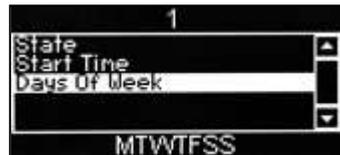
**N.B.** To select individual days, scroll through the menu using the ▲(up) or ▼(down) keys until the required day is highlighted.
