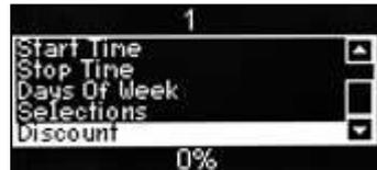
13. To enter the discount value, e.g. 50%, press the sequence 5-0 using the appropriate number keys on the drink selection keypad. Press the ↵ (Edit) key to return to the 11 (Discount) screen and verify that the status line displays the discount percentage value entered.
