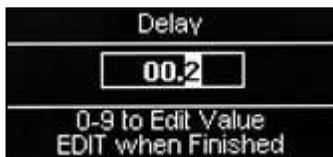
Press the ↵ (Edit) key and verify that the status line confirms that Delay (when highlighted) is set to 0.2hrs.
