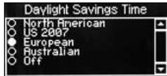
By default daylight savings time is set to Off. To choose one of the available options, press the ▲(up) or ▼(down) key until selected (indicated by the filled radio button) followed by the ↵ (Edit) key. Ensure that the required setting is displayed in the status line at the bottom of the screen.
