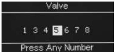
**Important:** Do **NOT** use this feature to test the valves feeding any Oltre brewers as they will not be in the sealed position and hot water will not be directed into the waste bucket.
