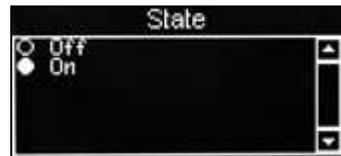
4. Press the ▼(down) key to highlight Event Type and press the ↵ (Edit) key to access the menu. Using the ▼(down) key, set the Event Type to Free Vend (indicated by the filled radio button). Press the ↵ (Edit) key to return to the Event 1 screen. Verify that the status line confirms the Event Type is set to Free Vend.
