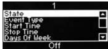
3. Press the ↵ (Edit) key to access the State sub menu. Using the ▼(down) key, set the state to On (indicated by the filled radio button). Press the ↵ (Edit) key to return to the Event 1 screen. Verify that the status line confirms the State is set to On.
