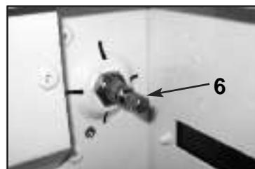
2. Remove the air intake cover (5) exposing the blanking plug. Access to this cover is made easier by first removing the B2C chute & cover (4). Remove the air intake blanking plug (6). Any remaining water will be ejected from the system.
