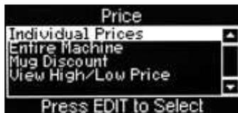
Certain programming functions require that the engineer chooses either one or multiple parameters within a sub program. These can take the form of either check boxes or radio buttons.
