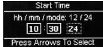
Press the ↵ (Edit) key to return to the Event 1 screen. Verify that the correct start time is displayed in the status line at the bottom of the screen.
