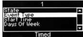
4. Press the ▼(down) key to highlight Start Time and press the ↵ (Edit) key. From this menu the operator sets the time at which the sanitation event will start. Using the drink selection keypad, press the sequence 0-7-0-0 to set the time. If necessary use the ▲(up) or ▼(down) key until AM appears in the dotted box.
