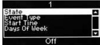
By default the current State is set to Off as indicated by the status line at the bottom of the screen.
