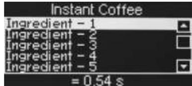
**NB.** Ingredient - 1 is the minimum throw of coffee; Ingredient - 3 is the normal throw of coffee and Ingredient - 5 is the maximum throw of coffee
