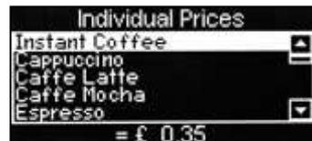
3. To change the price of the highlighted selection, press the ↵ (Edit) key. The LCD will change and display the screen as shown.
