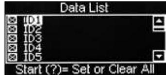
All data and events fields within a vending machine are assigned a unique code determined by the Standard. From this sub-menu the operator can choose to allow all fields to be available for download by pressing the START/? key or scrolling through the list and adding an X to the required fields.
