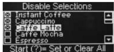
1. If necessary continue until all required drink selections have been checked. Pressing the X (Exit) key will move back to the Product Configuration screen and save the new parameters to the machines memory.
