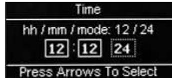
Press the ↵ (Edit) key to return to the Clock menu and save the new time. Confirm that the status line at the bottom of the screen displays the correct time when Time is highlighted.
