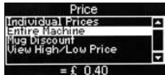
2. Press the ↵ (Edit) key to access the Entire Machine sub menu. To update the value, e.g. set a price of 50p, press the sequence 0-0-0-5-0 using the appropriate number keys on the drink selection keypad.
