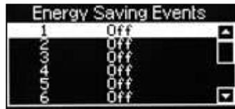
2. Press the ↵ (Edit) key to access the menu. The LCD will display the screen as shown. By default the current State is set to Off as indicated by the status line at the bottom of the screen.
