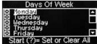
**N.B.** To select individual days, scroll through the menu using the ▲(up) or ▼(down) keys until the required day is highlighted. Press the ↵ (Edit) key to select the day, indicated by an X appearing in its adjacent box.
