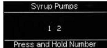
8. To prime syrup pump 1, press and hold button 1 on the drink selection keypad until the syrup appears from the dispense head. Repeat for syrup pump 2 by pressing and holding button 2 on the drink selection keypad. Press the X (Exit) key to return the machine to standby mode. Empty the waste bucket and refill to the machine.
