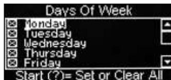
Using the ▼(down) key and the ↵ (Edit) key, highlight and select additional days of the week that the Energy Saving period will take place. When complete press the X (Exit) key to return to the Event 1 screen.
