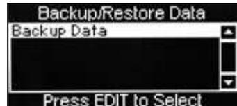
2. Press the  $\leftarrow$  (Edit) key to access the menu. The LCD will display the screen as shown. To backup the memory press the  $\leftarrow$  (Edit) key. After a few seconds the machine will beep once and the Initialising screen will be displayed before the machine returns to standby mode, ready to vend.
