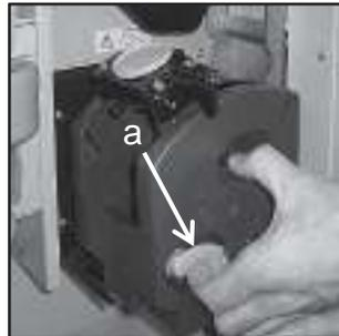
2. Carefully unclip the wiper arm from the brewer unit and place to one side.
