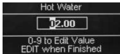
This is the length of time in seconds that the milk motor will run and can be changed by entering a new value and saving the new setting by pressing the Edit button
