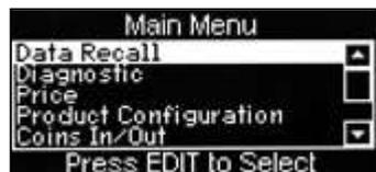
**N.B.** Coins In/Out will only be displayed on machines fitted with an MDB coin mech.
