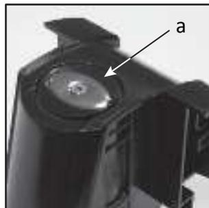
7. Ensure that the piston drive cam (b) is positioned as shown.
